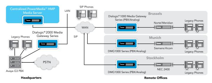
Figure 2. Converged IP Media Server Architecture
