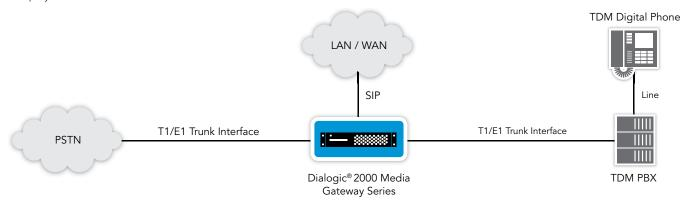
Figure 4. Access Gateway with Survivability Capabilities
